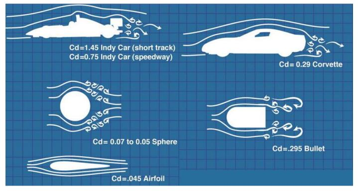
Any object moving through a fluid experiences drag - the net force in the direction of flow due to pressure and shear stress forces on the surface of the object.
